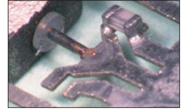
Anode, fuse and leadframe assembly
